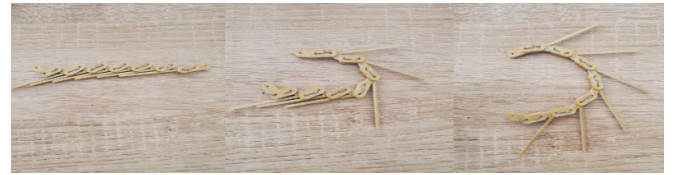
Fig. 6: A batwing mechanism, from left to right, undeployed, deployed around a small radius, and deployed around a large radius.
