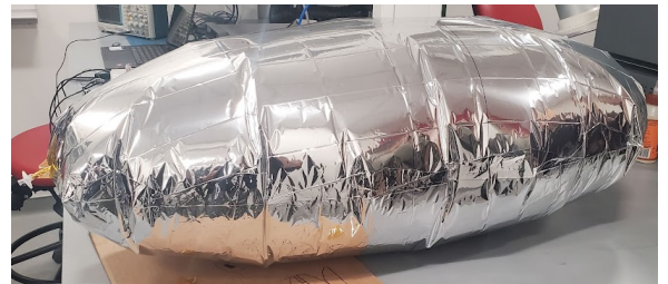
Fig. 3: Completed Lift Envelope with Luer Lock fill spout.
