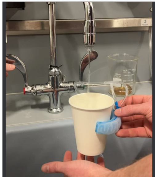
Fig. 10. Testing the grip strength of a leg by filling a cup with water
